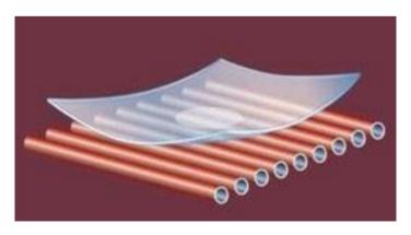
The only way to neutralise these defects is to balance the heating process by using additional heat transfer onto the upper surface. Significantly increasing the temperature of the roof does not resolve the problem because the low-emissivity coating will still reflect this increase in radiated energy. Moreover, this will cause the rollers to overheat which could aggravate the problem.
