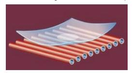
The only way to neutralize these defects is to balance the heating process by projecting additional heat onto the upper surface. Significantly increasing the temperature of the roof does not resolve the problem because the low-emissivity coating will still reflect this increase in radiated energy. Moreover, this will cause the rollers to overheat which could aggravate the problem.
