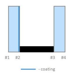
For Stopray T products coating must be in position #2 in DGUs and TGUs.
