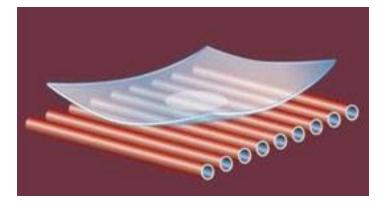
The only way to neutralize these defects is to balance the heating process by projecting additional heat onto the upper surface. Significantly increasing the temperature of the roof does not resolve the problem because the low-emissivity coating will still reflect this increase in radiated energy. Moreover, this will cause the rollers to overheat which could aggravate the problem.
